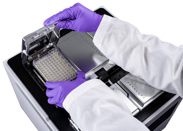
Figure 5. Locking an Agilent E-Plate View 96 into place with the locking clamp.
